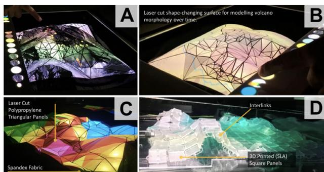
**Figure 2.** Semi-Solid laser cut surface [4] for modeling a shape-changing volcano morphology (A-B). Breakdown of laser cut semisolid surface structure (C). A 3D printed surface [5] used to show oceanography wave simulations (D-C).
