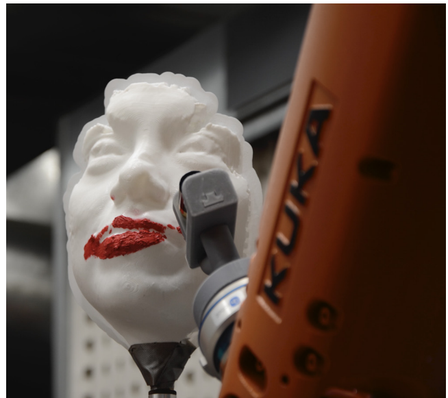
Figure 4: A photo of the real KR10 robot drawing lipstick on a 3D printed face.
