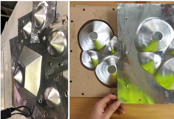
Figure 3: ISF testing pieces at RMIT in Melbourne and ARMHub in Brisbane.
