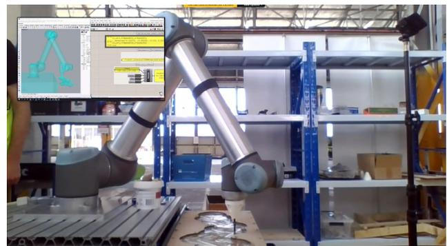
**Figure 1: UR10 collaborative robot ISF process in Brisbane and real-time digital twin being operated from several hundred km away in Melbourne.**
